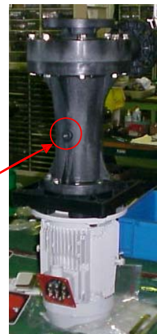
Air-release bolt with gasket
